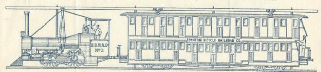
Engine A3. - 2 Cylinders 12x14. Weight 16 Tens, 400 Tens Traction.
