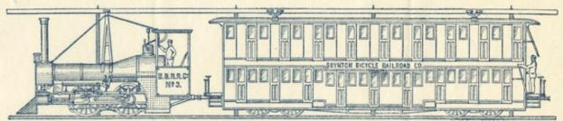
Engine M3. 2Cylinders 12x14." Weight 16 Tens, 400 Tens Traction, 550 Revolutions per Minute. 51/2 ft. Drivers. Speed: 100 Miles per hour.
