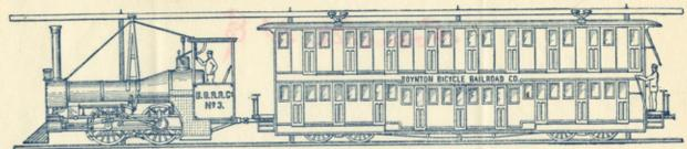
Engine M3. 2Cylinders 12x14. Weight 16 Tons, 400 Tons Traction.
