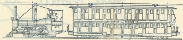
Engine M3. 2Cylinders 12x14. Weight 16 Tens, 400 Tens Tradition.
